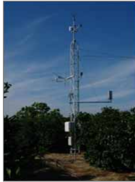
[Figure 7-9] Agricultural flux observation equipment installation (left: rice cultivation; right: tangerine cultivation)
