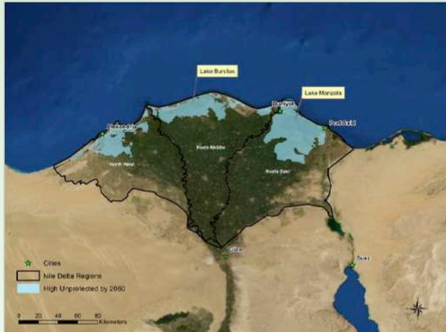
Fig (IV-1)-Projected inundation area including lakes of Maryut, Edku, Burullus and Manzala without any protection measures
